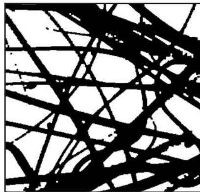
Figure 1 FIBER IMAGE USED FOR FIBER DIAMETER ANALYSIS
